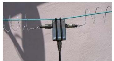
Here's a close-up of the feed point. The antenna is not self supporting so it is strung on a "messenger line" which is just a length of nylon cord stretched tight between two supports.
